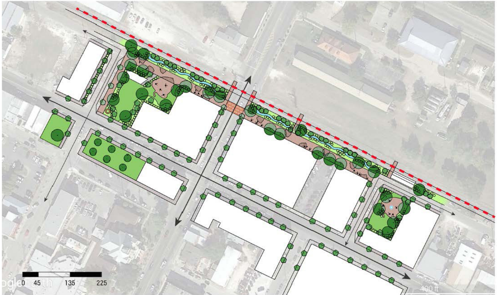
Conceptual plan featuring a restricted pedestrian access on Conner St., a series of gathering open spaces, bio-swales perpendicular to rail tracks and improved building facades and uses.
